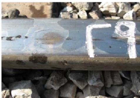
Figure 6. Lamination in rail in 49mm depth with 300 length
