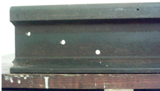
Figure 2. The manufactured calibration block
