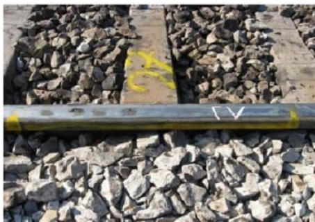
Figure 6. Lamination in rail in 49mm depth with 300 length
